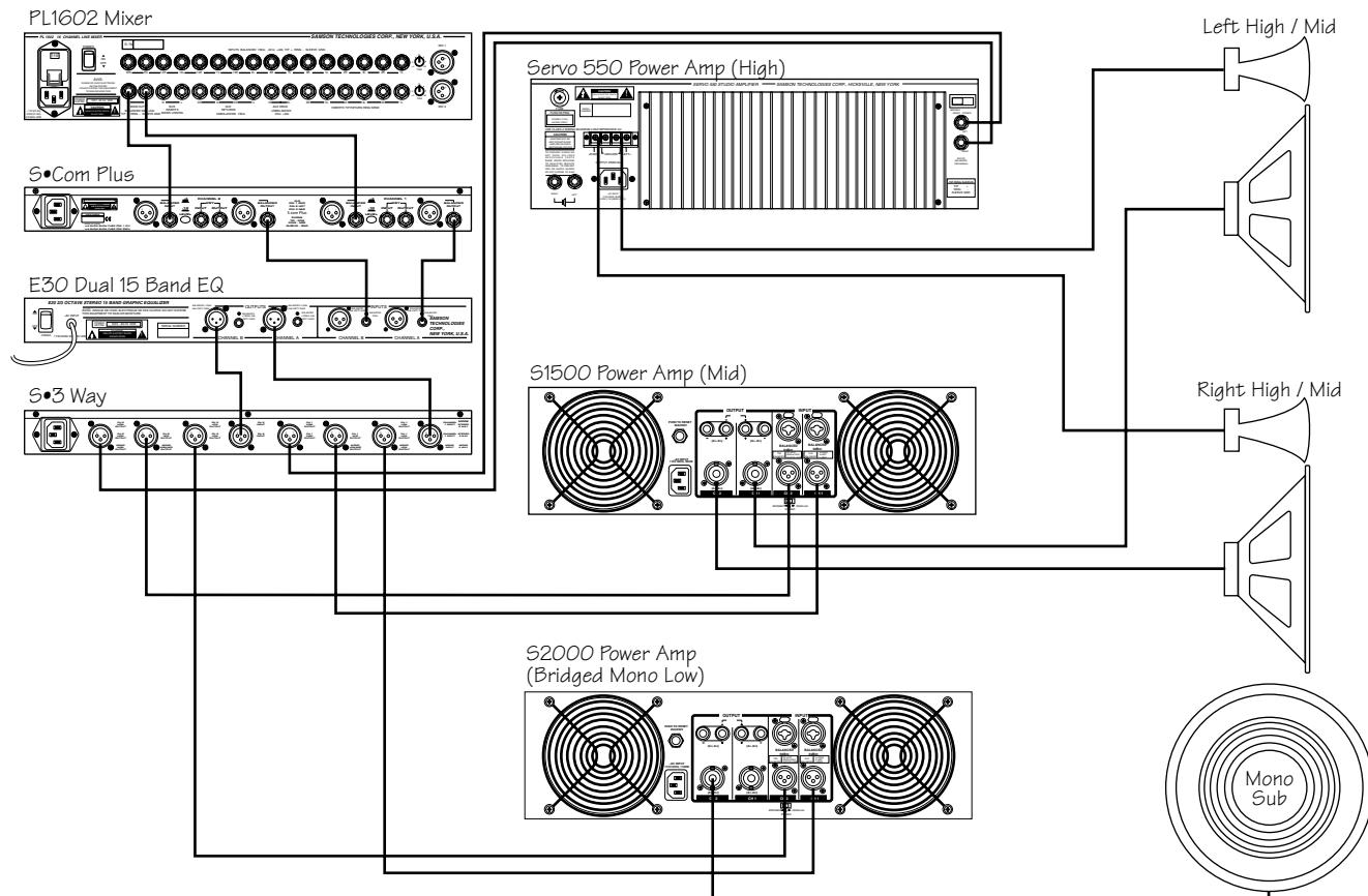
In this example, the S•com plus is inserted after the mixer and before the graphic equalizer, thereby compressing the full range signal from the mixer.
