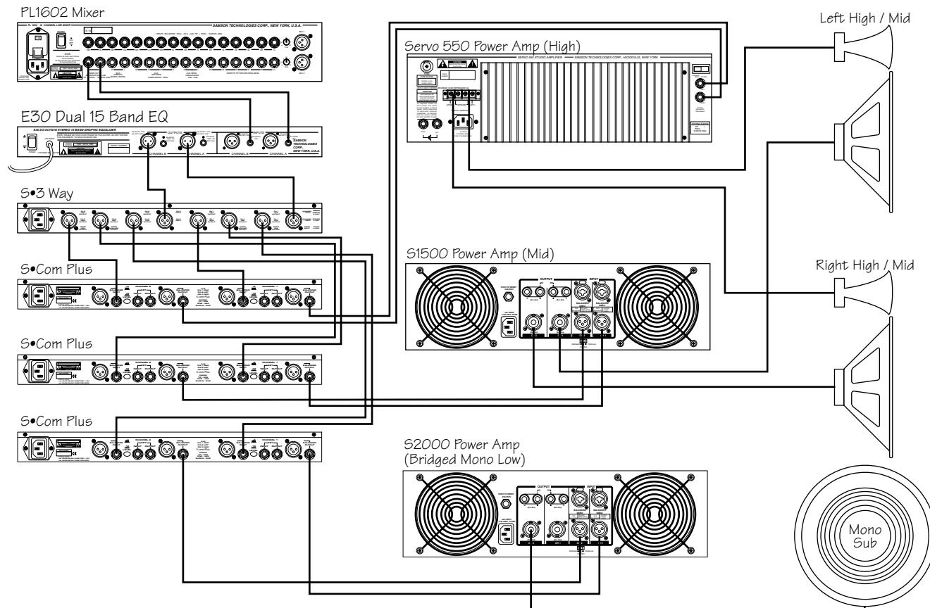
*In this example, three S•com plus' are inserted after the mixer, equalizer and crossover, thereby providing individual compression on the low, mid and high frequencies.*
