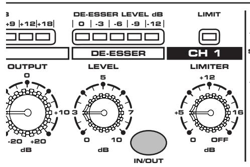
**Note: For Detailed De-Essing** - Since the Compressor and DE-ESSER share the same ATTACK and RELEASE settings you may consider using one of the S•com plus' channels exclusively for DE-ESSING. Experiment with fast ATTACK and RELEASE times when using the channel for DE-ESSING only.
